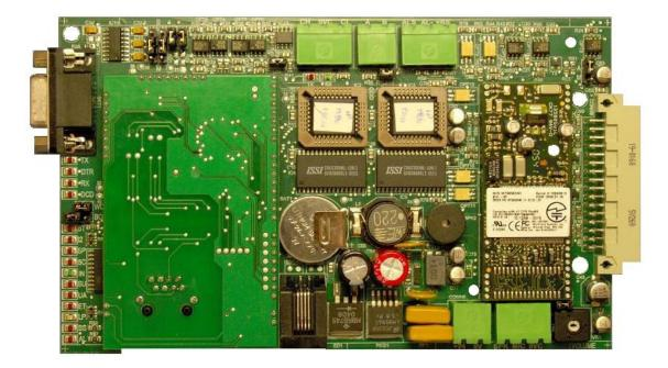
5.5) IP Board with Ethernet and GSM Modem
