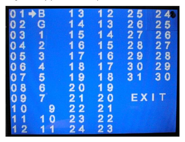
To select a floor to change use the 'scroll' keys to point at that floor, then press 'enter' and you will be passed to the floor set-up screen.
