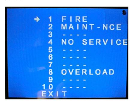
To change a message first select it with the +/- keys to move the arrow up and down. Then scroll through the available messages with the enter key.
